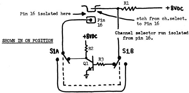
Parts: all resistors are 10K for MB8719, 5K for an 858 at 5V logic. Q1 is either a 2N3904 or 2N2222. Switch is DPDT.
