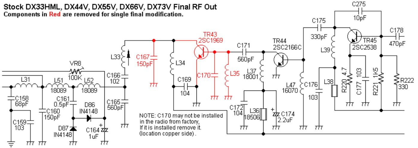
Stock DX33HML, DX44V, DX55V, DX66V, DX73V Final RF Out
