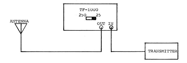
If your station utilizes an amplifier who's output is greater than 250 watts, the TF-1000 must be placed between the transmitter and amplifier. The power level switch must be placed in the position appropriate to your transmitter's output power.
