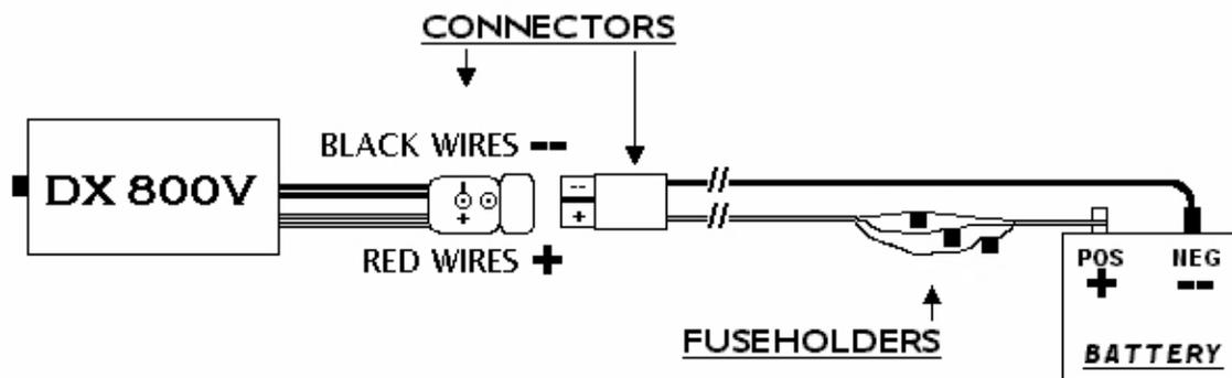
1. Install a 30 Amp ATC fuse into each Bussmann HHD fuseholder.
