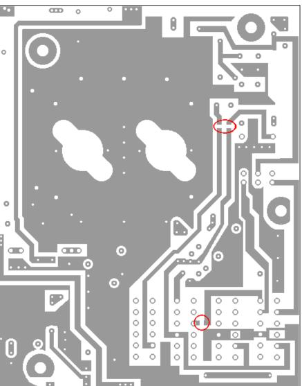
Note: The Driver PCB is a modified DX350V PCB all trace cuts are shown circled in Red above.
