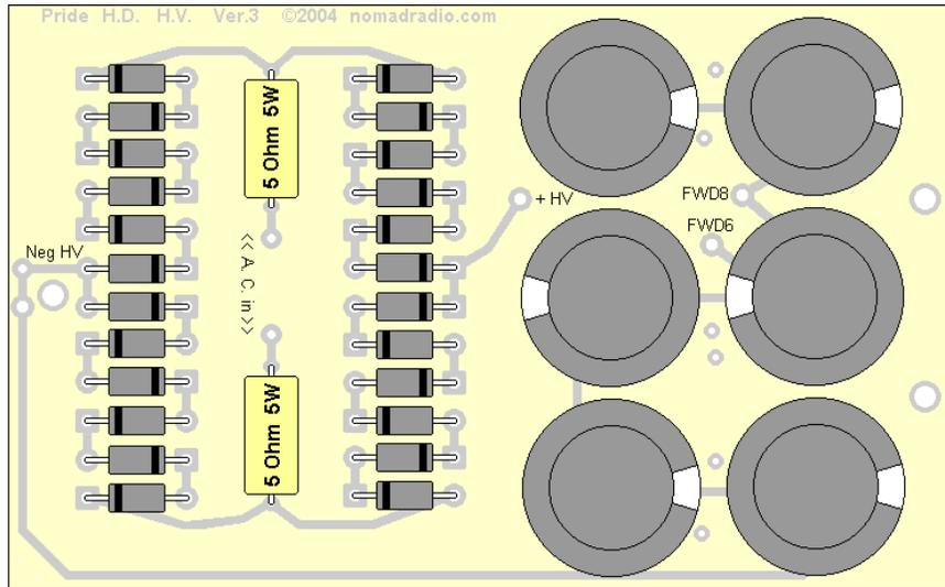
The Kit includes all the parts to build a single PCB HV Power Supply that replaces both HV PCB in a Pride DX300. This PCB lets you completely remove the original two H.V. circuit boards and install the single-piece replacement.
