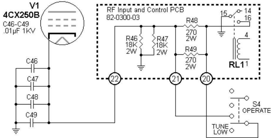
Figure 3-41 Cathode Circuit
