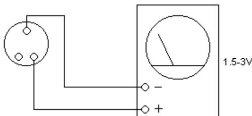
Figure 4-0 Meter Connection
