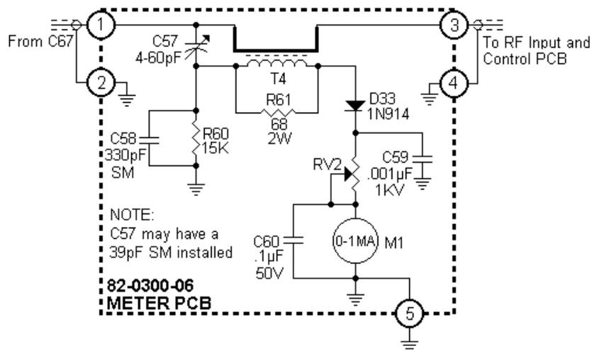
Figure 3-6 Wattmeter Circuit
