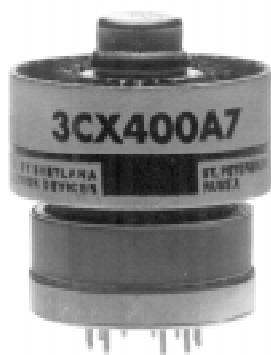
**T**he Svetlana™ 3CX400A7/8874 is a high performance ceramic/metal power triode designed for use in communications, paging and commercial service. The principal use is as an RF amplifier, in Class A, B or C service. The Svetlana 3CX400A7/8874 may also be operated as a pulse modulator with an increase in maximum plate voltage up to 3500 volts. Maximum plate current is 6 amps at a pulse duration of 100 microseconds.
